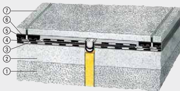
① Deck ② Lightweight concrete ③ Membrane ④ Elastic joint ⑤ Membrane ⑥ ITALPROFILI support ⑦ Paving slabs
